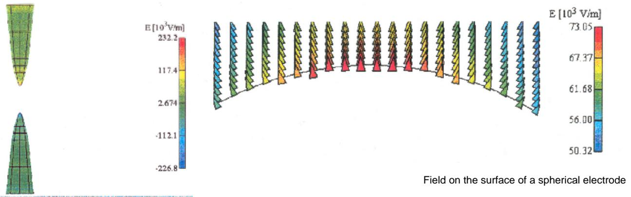
Potential distribution on the surface of 2 needle electrodes
