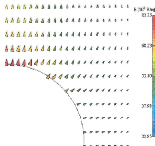
Field between 2 spherical electrodes (quarter of the symmetry)
