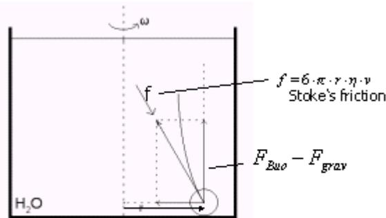
When the liquid is rotating the same forces act. There is, however, one new force acting which is the centripetal force. This force makes the ball moving towards the axis of rotation.
