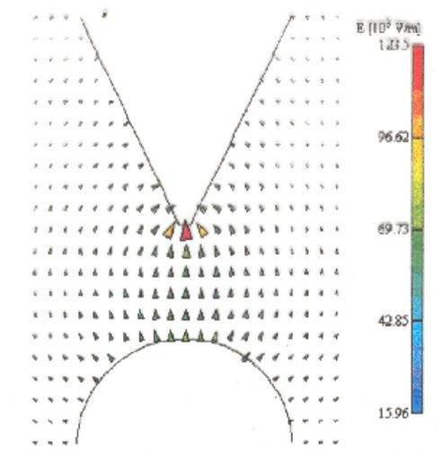
Electric field between a spherical and a point electrode
