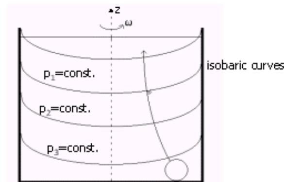
When the liquid is rotating the former plane isobarics become parabolic.
